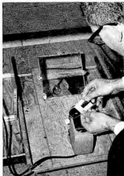
Fig. 2. Film clip is inserted into holder.
